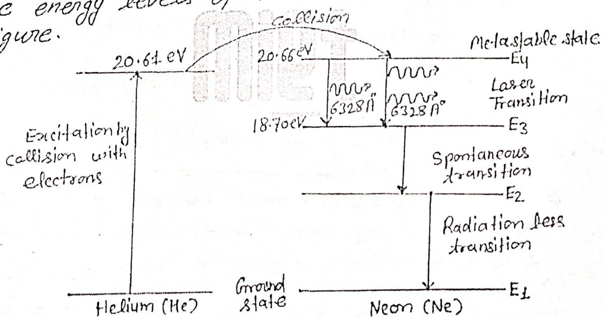
When an electric discharge passes through gas, the electrons in discharge tube collide with He and Ne atoms as He atoms are lighter than the Ne atoms they are easily excite to metastable state 20.61 eV and Ne atom to 20.66 eV respectively above the ground state. Some of excited He atoms transfer their energy to unexcited Ne atoms by
