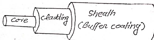
second layer (cladding). Its refractive index is slightly more than cladding.
