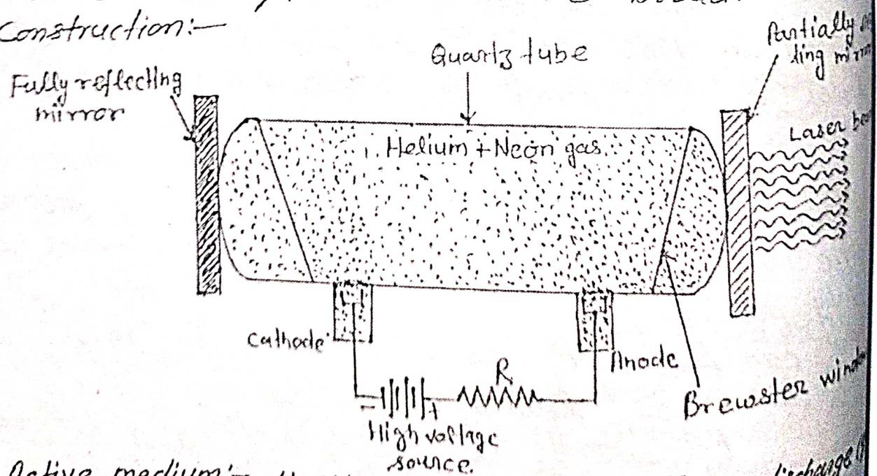
Active medium:- He-Ne laser consists of a discharge tube containing the Helium and Neon in the ratio 7:1 at a total pressure of about 1 torr (1mmHg).
