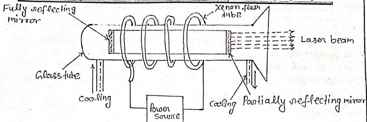
Ruby rod is surrounded by a helical xenon flash tube, which provides light to raise chromium ions to upper energy levels.
